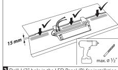
2 Drill I/2" hole in the LED Panel (B) for installation of LED/test switch on indicated area.
