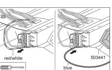
4 Disconnect the red/white single wire from the EvoKit driver. Replace it with the blue output wire from the 503441 (Z). Place a wire nut over the original red/white wire for proper isolation.
