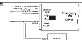
7a Emergency LED driver wiring in combination with **0-10V** and MK 10 version
