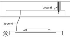
10a Situation 1 Grounding: Screw grounding cable from Led Panel (B) to original troffer if host fixture ground connection is made trough host fixture.
