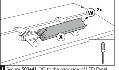
Secure 503441 (X) to the back side of LED Panel (B) using two screws (W).
