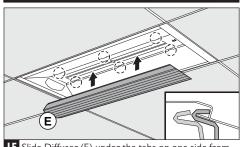
15 Slide Diffuser (E) under the tabs on one side from either Panel and press diffuser (E) over the tabs on opposite panel. The installation is now complete.
