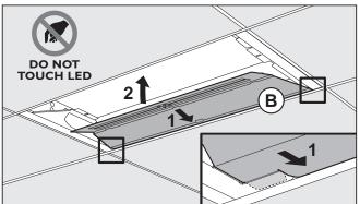
7 Install SR LED panel (B) in between troffer and T-grid, making sure the tabs at each corner of the LED panel slide into the respective slots on the side panel.
