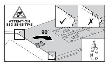
8 Push LED panel upward into position so that the tabs sits above the side panels (this may require a push up on the tabs while pushing outward on the side panels). Fixate panels and establish ground by turning each fastener 90 degrees.
