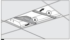
5 Install Side panels (A) in-between troffer and T-grid.
