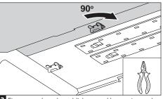
13 Fixate panels and establish ground by turning each fastener 90 degrees.
